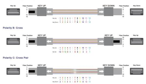
Note: MPO-12 (Male) on the rear. APC for G.657A fibres, UPC for OM4 fibres
