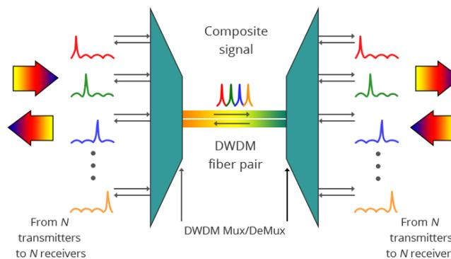
Active DWDM systems normally utilizes transponders and muxponders to 'translate' various low order client signals into DWDM channel specific signals with higher bitrate bandwidth.
