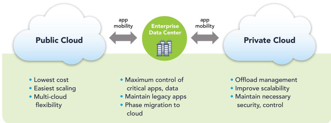
**Figure 1:** Advantages of Different Infrastructures in a Hybrid Cloud
